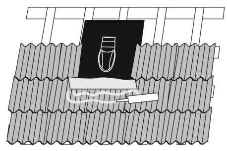
Push the bottom edge of the flashing down firmly.
